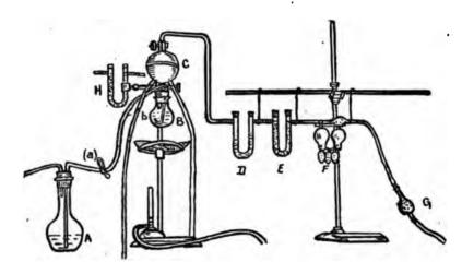
When the apparatus is ready, weigh out into the flask (B) about 0.8 gram of the dolomite and cover it with 15 cc. of water. Carefully wipe the Geissler bulb (F), with its calcium chloride prolong tube, and weigh accurately. Afterward stopper the openings by means of small pieces of rubber tubing closed by pieces of glass rod.
